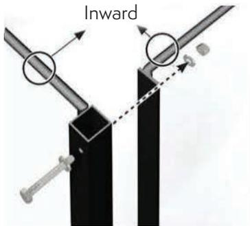
Ensure the RODS are facing inward. Secure with 1/4" BOLTS, WASHERS & LOCKING NUTS
